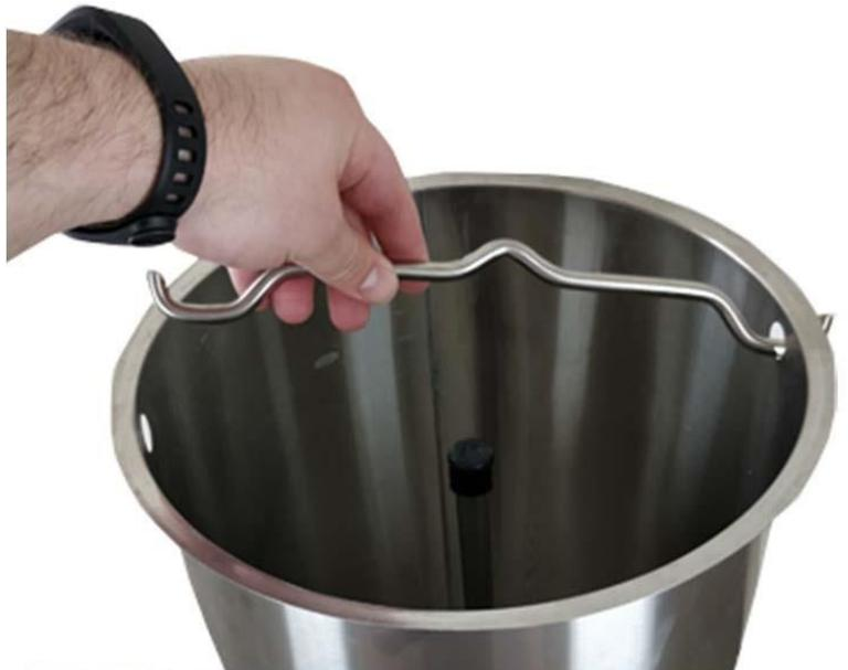
Once the handle has been fitted you can lift/maneuver the malt pipe easily.
