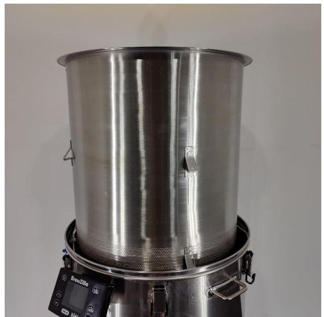
Once the malt pipe is suspended above the boiler and is securely supported by the halo ring then pour warm water (approximately 75-80°C) onto the top screen inside the malt pipe to rinse the grain of the majority of the remaining sugars. This process will probably require 5-15 Liters of water depending on your recipe and desired gravity that you are trying to achieve.
