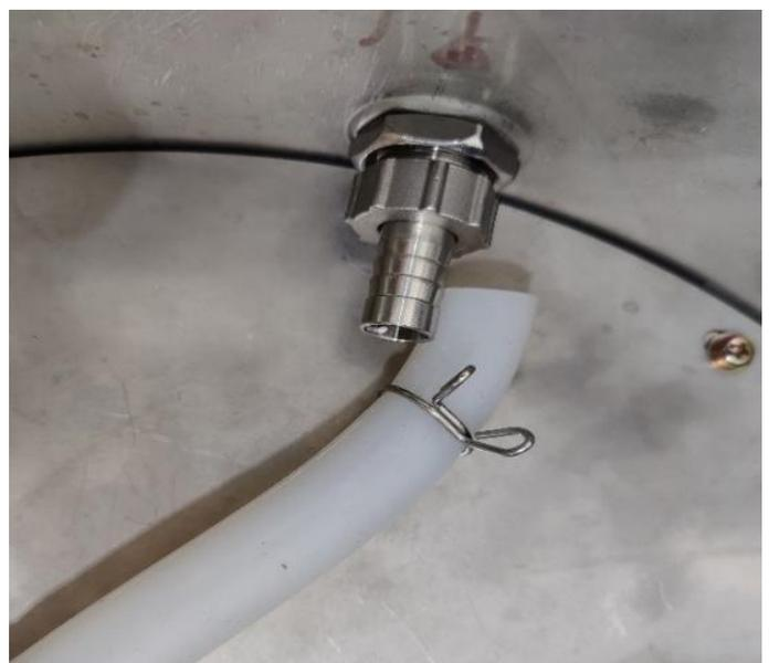
Push the unconnected silicone hose from the pump over the barb on the tap and secure in place with the wire clamp.
