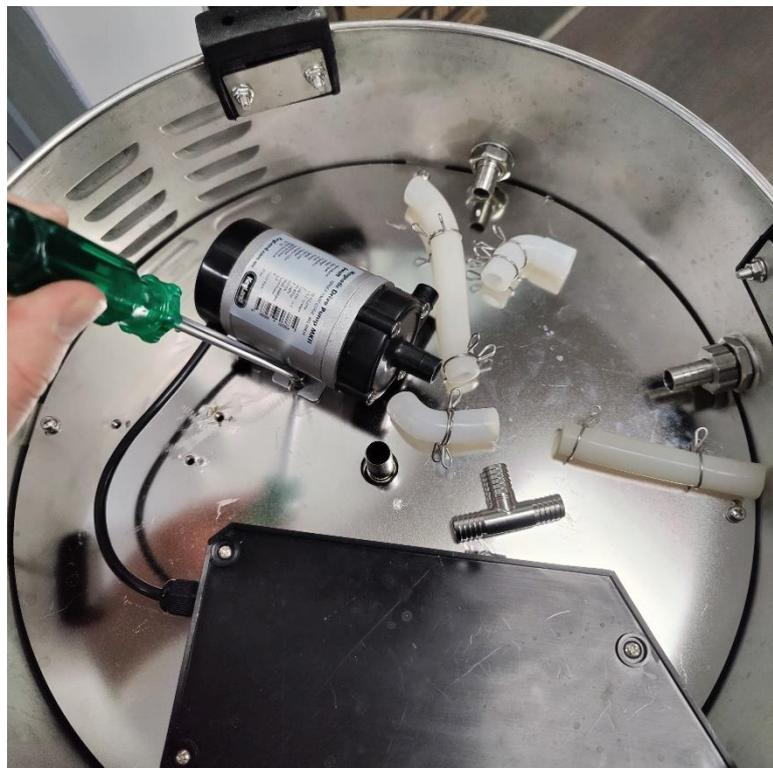
Then change the pipe work as shown below such that the tee piece from the boiler outlet splits to the tap before it reaches the pump inlet.
