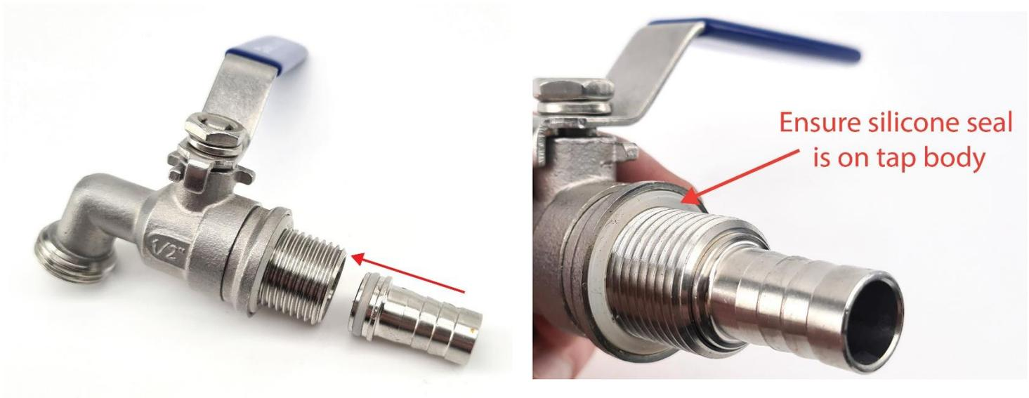
Then turn the BrewZilla upside down and insert the thread of the tap through the pre-drilled hole in the boiler. Secure the tap on the inside of the boiler using the hex nut and secure the barb in place by tightening the retaining nut onto the taps thread.
