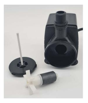
**Step 5.** The impeller cavity can be cleaned with a soft toothbrush or cloth.
