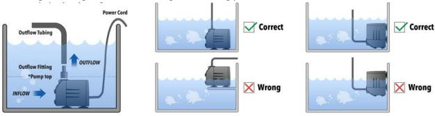
The pump can either be setup in the bucket for portable use or in a sink for easy clean up.
