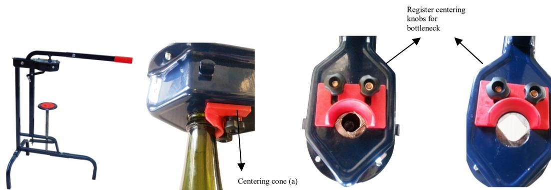
With **adjustment of the level of insertion of the cap** and centering cone (a) which allows the **reduction of the inlet hole** and ensures **optimal alignment of the cap with the bottle**. Ideal for natural champagne corks  $\varnothing$  max 30.5 mm x h max 48 mm and bottles with a minimum height of 23 cm, maximum 34 cm. Preset for crown cap device  $\varnothing$  26 or 29 mm and bottles with a minimum height of 17 cm, maximum 28 cm.
