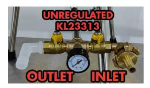
**Step 9.** Note: We will be Installing the Water Regulator to the stock standard outlet drainage port. The right-hand side inlet port will now become your outlet drainage port. For more information on how to install this inline regulator please see below.
