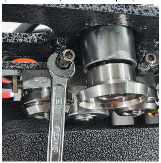
3. Insert a 5mm Allen key into the socket of the bump stop adjustment screw and adjust the amount of thread showing to change the 1st Op roller gap "X"
