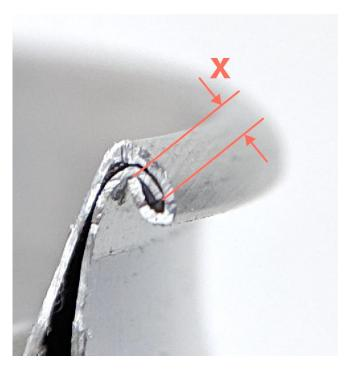
If you determine that the actual overlap between the can body and can end is less than 0.4mm following the first operation, make sure that your 1st operation roller is in the correct position.
