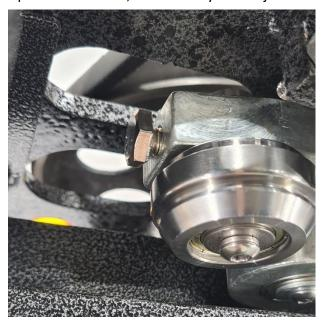
4. Slide the roller vertically along the drive shaft to set the gap "Y" at 0.05 mm. The best results can be achieved when the 1<sup>st</sup> operation roller is as close as possible to chuck in the y-axis without touching the chuck. Ensure that the gap "Y" is measured from the flat face of the roller to the top of the chuck (as shown below).
