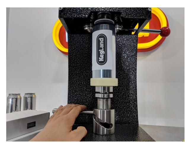
**NOTE:** The quality of the seam is greatly dependent on the can coming in contact with the chuck concentrically.
