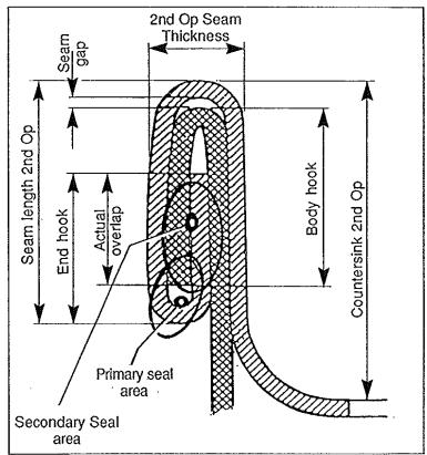
The forming of the 1<sup>st</sup> operation seam is the most important operation as this operation takes the end curl and can flange and begins the forming process. It's the formation/dimension of this 1<sup>st</sup> seam that controls the effectiveness of the 2nd operation seaming roll profile in achieving a hermetic seal.
