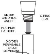
remove any stains without damaging the platinum tip.
