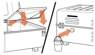
**NOTE:** Be sure the grease drain spout on the grease drip tray extends through the opening in the back of the grill.
