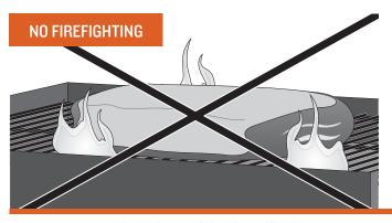
No more worrying about drippings flaring up and causing those nasty fireballs that destroy your meal. Traeger Wood Fired Grills are designed to cook by using indirect heat. All drippings are safely channeled into an external grease pan for easy disposal.
