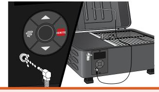
Insert the meat probe's plug into the socket on the lower left corner of the controller, then route the probe cable through the notch in the grill front, as shown.
