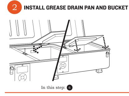
**NOTE:** Be sure the grease drain spout on the grease drain pan extends through the opening in the back of the grill. **IMPORTANT:** Always be sure to position the grease drain bucket under the spout during use!
