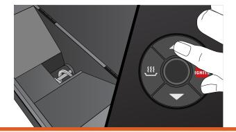
Make sure there are no foreign objects in the auger. With the grill in Idle mode, press and hold the UP and IGNITE buttons simultaneously. The display will flash "Pri" and the auger will begin priming.
