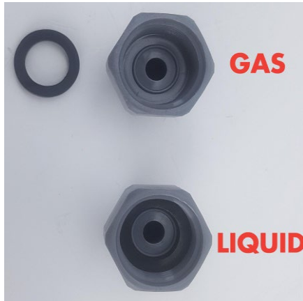
Remove 5/8 EPDM washer from gas 5/8" duotight
